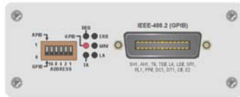
Rear-panel DIP switch set DOWN to select GPIB control.
